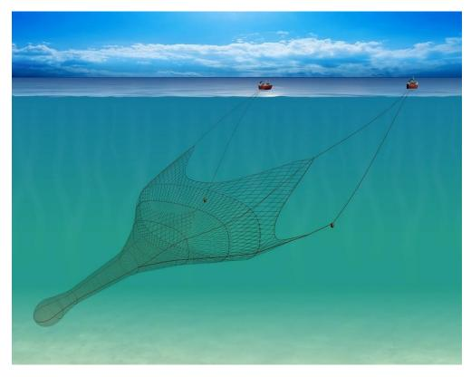
Figure 17 - Pelagic pair trawl (Seafish, 2020c, <u>https://seafish.org/gear-database/gear/pelagic-pair-trawl/</u>[unedited]).
