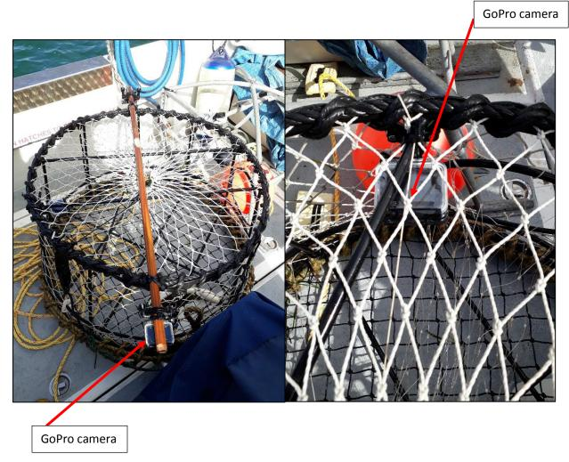
Figure 1 GoPro set up on cuttle pot
