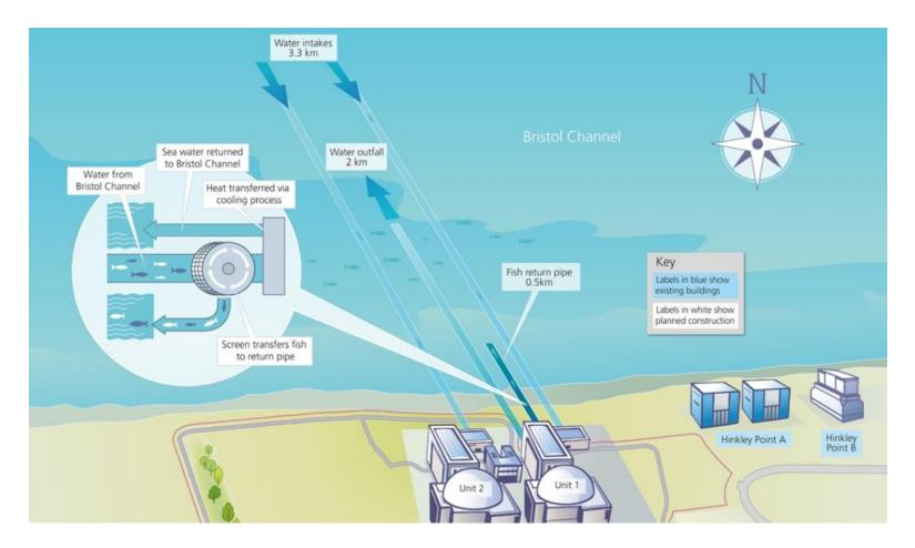
The illustration below was used in The Times article on 20<sup>th</sup> July 2019 on Hinkley Point C water intake system and the impact it may have on fish population in the Severn Estuary. The full Times article can be read <u>here.</u>
