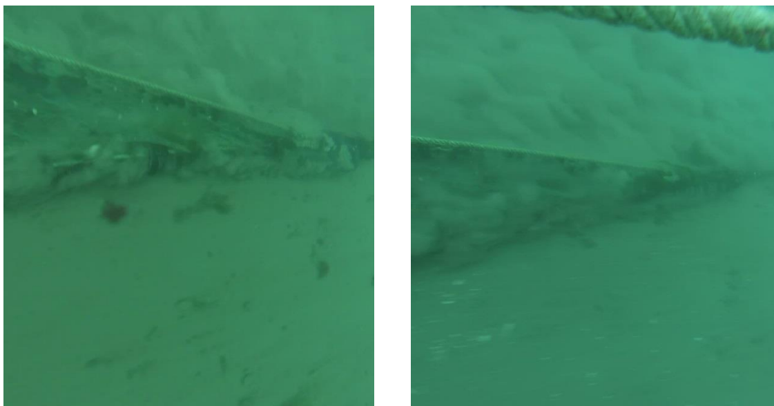
Figure 2 Sediment plume caused by footrope on heavy trawl gear
