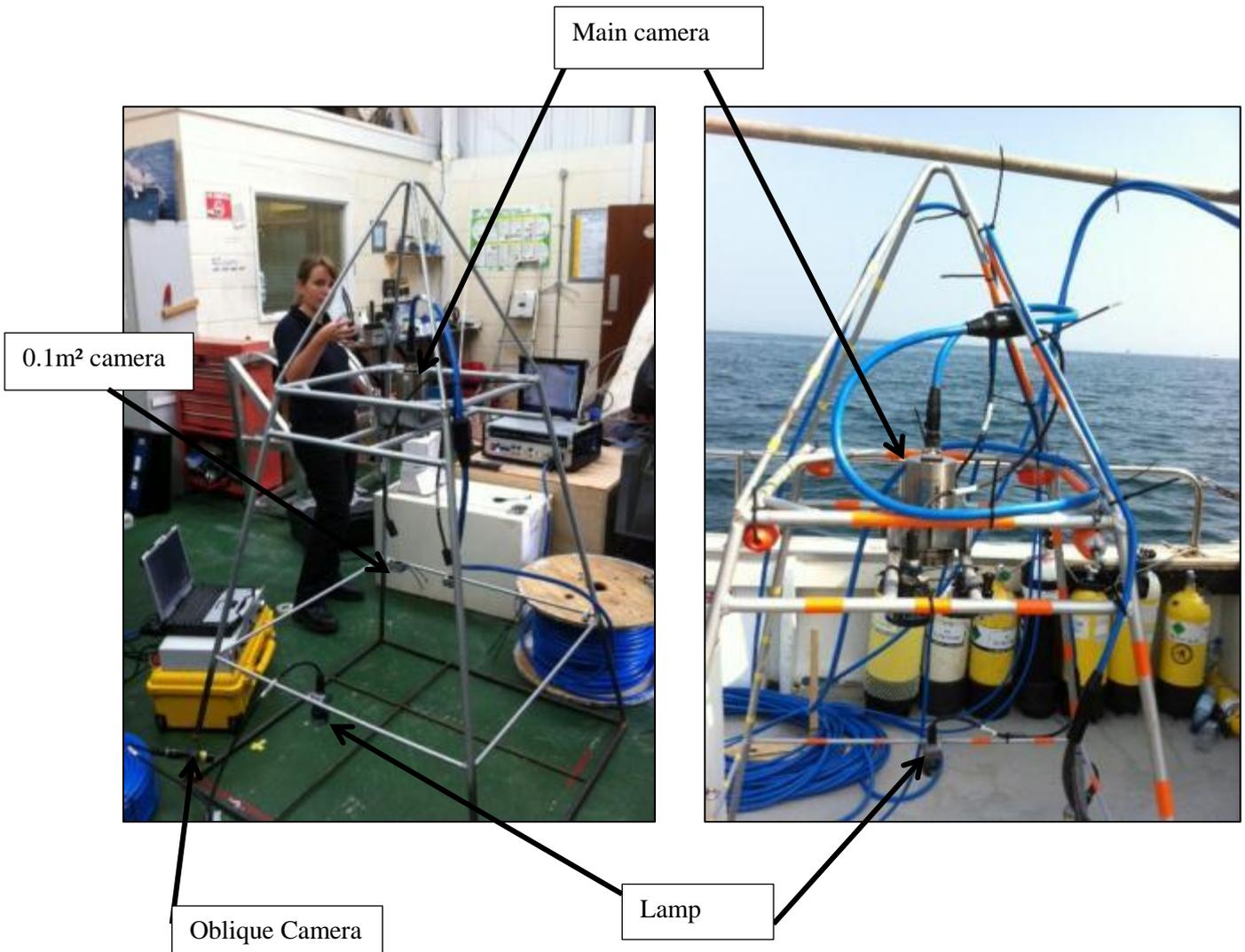
Figure 20. Pyramid frame set up.
