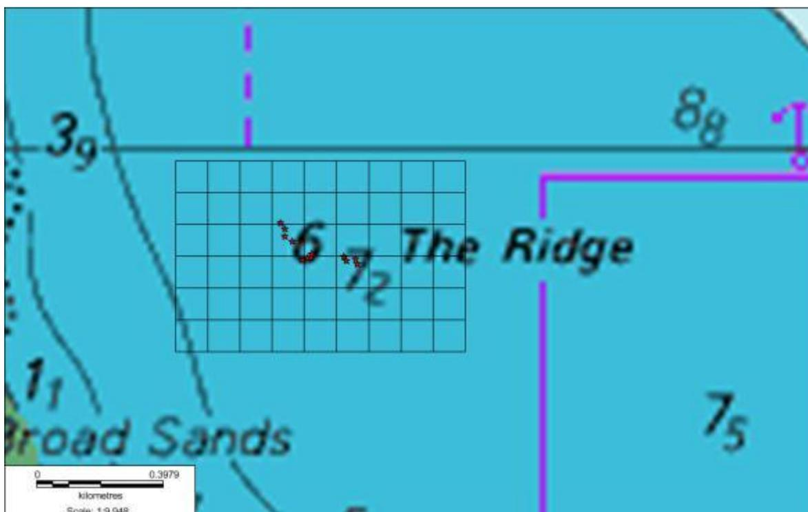
Figure 24. Example of grid made in MapInfo.
