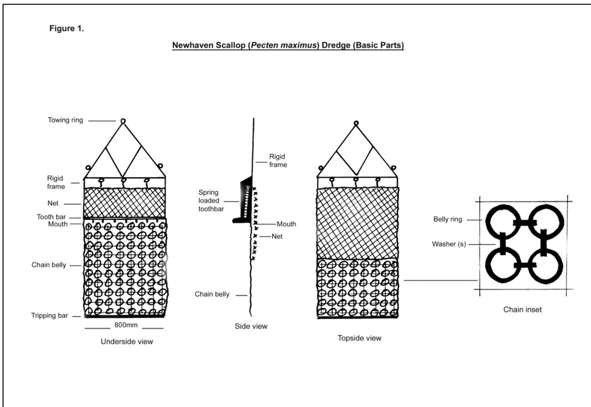
Figure 5 Schematic of Newhaven dredge (Hughes, 2009)
