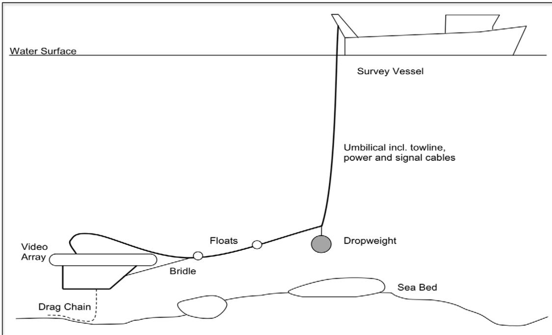
Figure 22. Schematic of array in use (Sheehan et al, 2010.)
