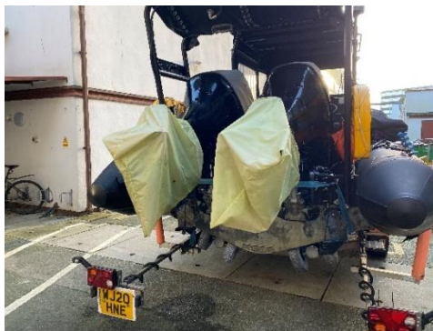
Figure 5 Extended light boars for driving and propeller covers fitted
