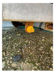
Figure 11 PV Enforcer Wheel bearing flush valve 2
