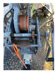
Figure 5 PV Enforcer Winch handle disengaged
