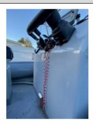
Figure 4 PV Enforcer Console kill cords in place
