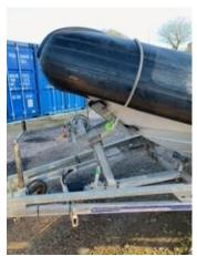
Figure 9 PV Enforcer bow liner over winch for launching (sideview)
