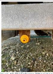
Figure 10 PV Enforcer Wheel bearing flush valve 1
