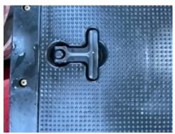
Figure 14 Battery locker catch closed
