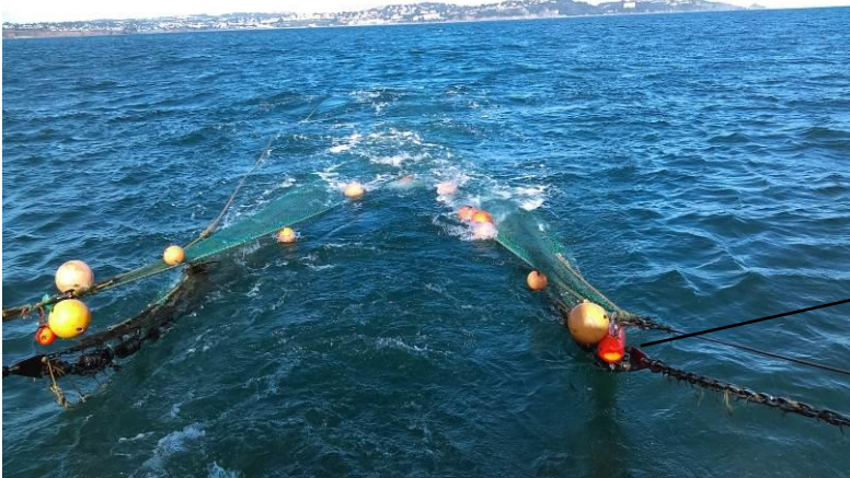
Orange Scanmar sensors attached to the wing ends of the trawl
