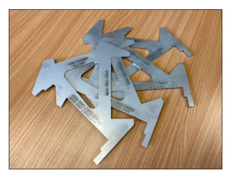
D&S IFCA has introduced Minimum Conservation Reference Sizes (MCRS) for selected shellfish within its District. To assist fishers to remain compliant with the legislation, new gauges have been produced that are locally made from 316 stainless steel and will be of use to measure the following species:
