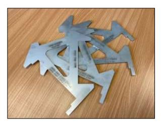
D&S IFCA has introduced Minimum Conservation Reference Sizes (MCRS) for selected shellfish within its District. To assist fishers to remain compliant with the legislation, gauges have been produced that are locally made from 316 stainless steel and will be of use to measure the following species:
