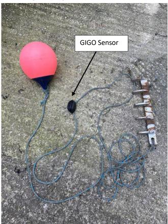
Prior to the sea trails undertaken on 2<sup>nd</sup> February 2024, Officers fitted the new Succorfish IVMS device that had already been paired to the four gear in gear out sensors. The sensors are only paired to one device and would not be detected if used on another vessel with a different IVMS device.
